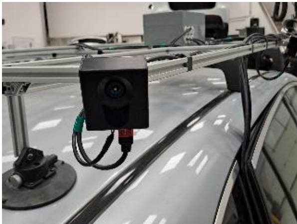
Figure 7. ToF camera mounted on roof
