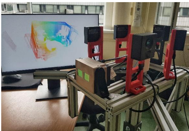
Figure 21. AI-based near field, high resolution 360-degree perception system's mobile setup used for initial testing, verification and algorithm design.
