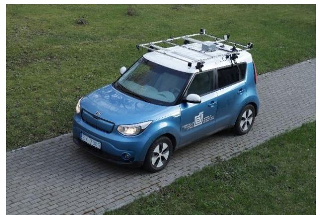
Figure 22. Perception system's integration onto EDI's Drive-by-Wire vehicle.
